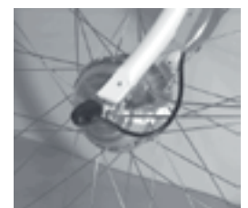
Motor in the front wheel.
