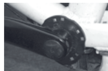
Sensors in the crankshaft.
